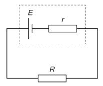
What is the maximum value of *E* if the resistor does not overheat?
