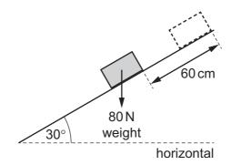
What is the work  $W_g$  done against the gravitational force and the work  $W_f$  done against the frictional force?
