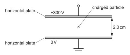
The acceleration of the particle is  $7.15\times10^{11}\,m\,s^{-2}$  downwards. The particle has a mass of  $3.34\times10^{-27}\,kg$ .
